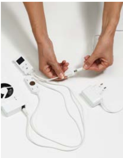
Fig. 11 – Connecting the Control Sensor (F) and the power adapter (D).
